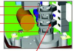
Place 2 mm Allen wrench in position to adjust cams.
