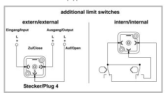
Pin 1 = Input (+/L) Pin 2 = output "close" (+/L) Pin 3 = output "open" (+/L)
