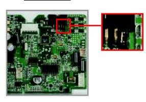
Jumper plugged Jumper removed
