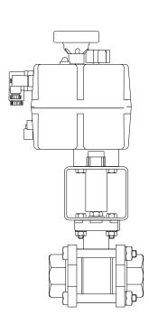
Assembling with bracket and adapter
