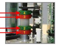
To ensure that the position confirmation works, adjust the confirmation cams (3 & 4) 3° (+/-1°) before the motor stop. To avoid problems, you should adjust the cams 3 and 4 always about 3 degrees before the engine shut-down.
